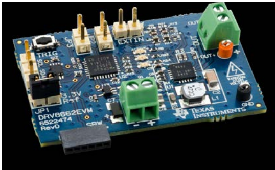
Fig 2. DRV8662EVM haptics driver module.
